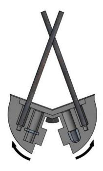
To remove the recess former, insert two rods in holes  $\bf C$  and move towards each other. Do not use a hammer to remove the recess former as that may destroy the former.
